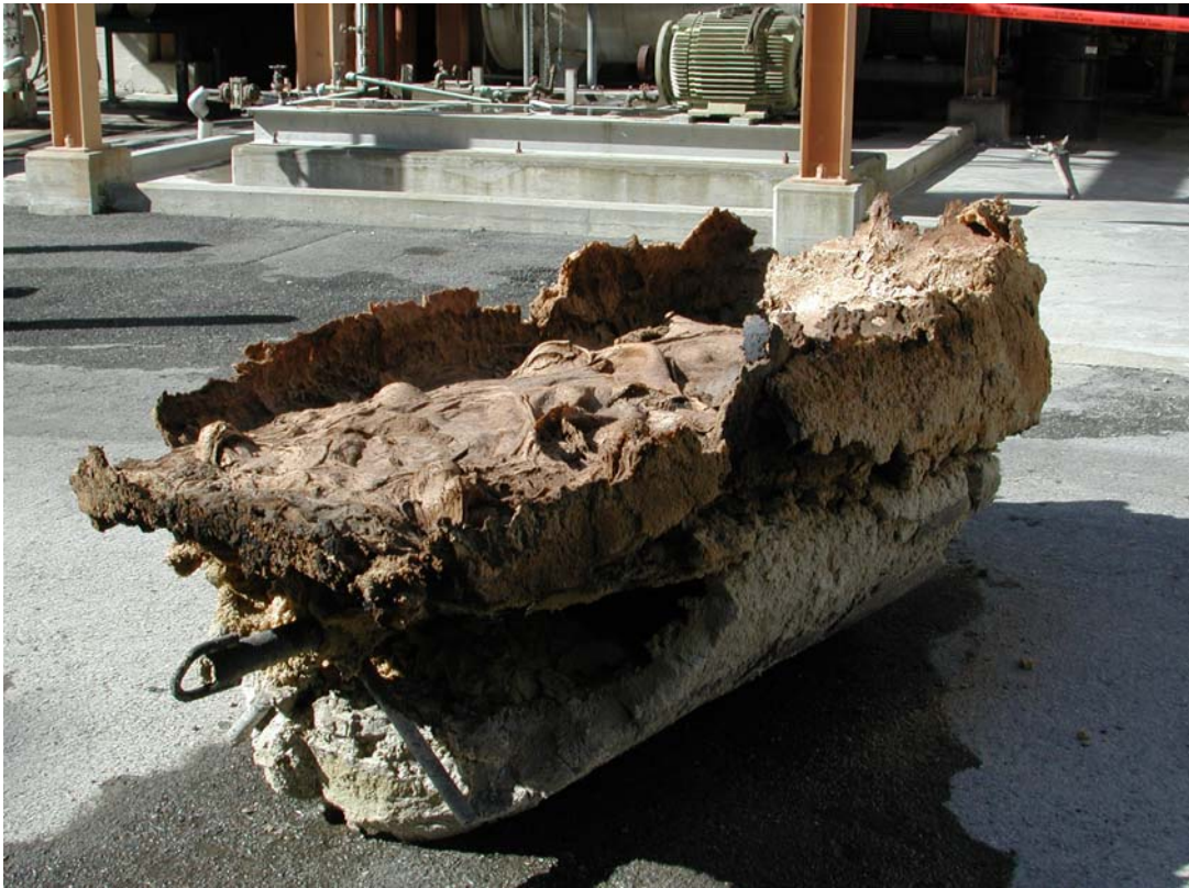
Figure A-6. Material extracted from the polymer catch tank on March 11, prior to the incident.
